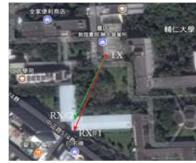
Fig. 2. The location of the transmitter (TX) and the receivers (RX#1 and RX#2). The horizontal distance between the TX and the RX #1 (RX #2) is 110 meters (100 meters). The TX and the both RXs (RX #1 and RX #2), respectively, with a height of 24 meters and 1 meter above the ground level.
