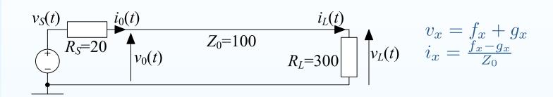
From Ohm's law at x = 0, we have  $v_0(t) = v_S(t) - i_0(t)R_S$  where  $R_S$  is the Thévenin resistance of the voltage source.
