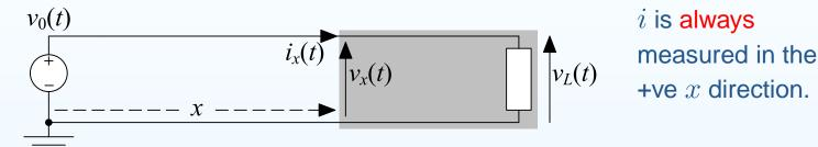
Then  $v_x(t) = f_x(t) + g_x(t)$  and  $i_x(t) = Z_0^{-1} (f_x(t) - g_x(t))$ . Note: Knowing the waveform  $f_x(t)$  or  $g_x(t)$  at any position x, tells you it at all other positions:  $f_y(t) = f_x (t - \frac{y-x}{u})$  and  $g_y(t) = g_x (t + \frac{y-x}{u})$ .
