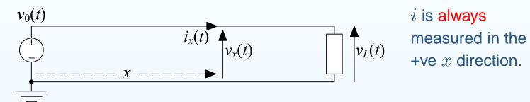
Then  $v_x(t) = f_x(t) + g_x(t)$  and  $i_x(t) = Z_0^{-1} (f_x(t) - g_x(t))$ . Note: Knowing the waveform  $f_x(t)$  or  $g_x(t)$  at any position x, tells you it at all other positions:  $f_y(t) = f_x \left(t - \frac{y-x}{u}\right)$  and  $g_y(t) = g_x \left(t + \frac{y-x}{u}\right)$ .
