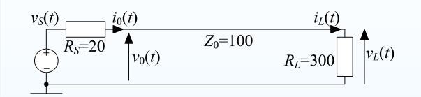
From Ohm's law at x = 0, we have  $v_0(t) = v_S(t) - i_0(t)R_S$  where  $R_S$  is the Thévenin resistance of the voltage source.
