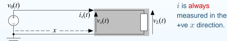
Then  $v_x(t) = f_x(t) + g_x(t)$  and  $i_x(t) = Z_0^{-1} (f_x(t) - g_x(t))$ . Note: Knowing the waveform  $f_x(t)$  or  $g_x(t)$  at any position x, tells you it at all other positions:  $f_y(t) = f_x \left(t - \frac{y-x}{u}\right)$  and  $g_y(t) = g_x \left(t + \frac{y-x}{u}\right)$ .
